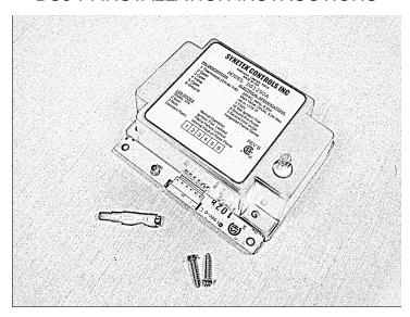
Synetek Controls Inc. model DS3-F replaces the following 24VAC Direct Spark Ignition controls in commercial laundry dryers. The Model DS3-A is designed for simple installation and long lasting operation by eliminating most nuisance lockouts and providing simple diagnostic indication of failure.
